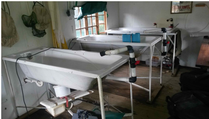
Figure 2.2: Mbona incubator baths have one California type tray (size: 0.5 \text{ m} \times 0.4 \text{ m} = 0.2 \text{ m}^2 ). When hatching trays are removed, the bath is used for rearing the fry.
